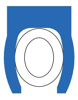
Spring energized flange seal for internal pressure
