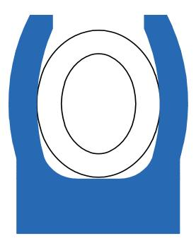
Spring energized flange seal for external pressure
